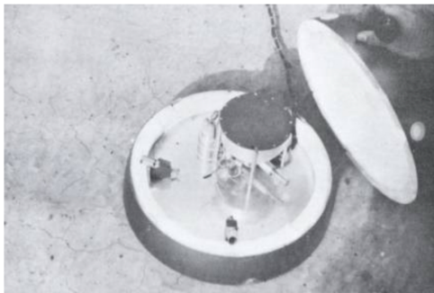
FIG. 2. Mark III Gulliver in simulated planetary lander capsule. Projectiles fire through the assembled housing. Note that opposite end of unit is up compared to Fig. 1. Instrument operates in any position.
